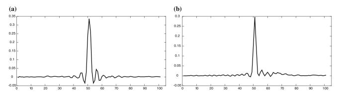
Fig. 13 Spatial convolution kernels for real sequences provided by INA, P = 101 (a) Tachan sequence, (b) Au théâtre ce soir sequence
