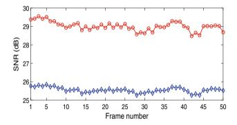
**Fig. 2 Foreman** sequence: SNR values per frame : Degraded (*blue diamond*), restored (*red circle*) (Color figure online)
