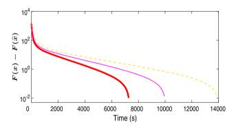
**Fig. 5** Comparison of the preconditioning strategies in terms of execution time (s.): preconditioning strategy (69) (*solid tick red*), no preconditioning strategy (68) with exact norms (*solid thin magenta*) and no preconditioning strategy (68) with approximated norms (*dashed thin yellow*) (Color figure online)
