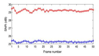
Fig. 3 Claire sequence: SNR values per frame : Degraded (*blue dia-mond*), restored (*red circle*) (Color figure online)
