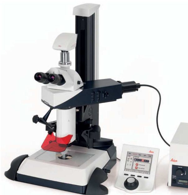
Fig. 1. A commercial MACROscope, the Leica MacroFluo TM Z16APO.
