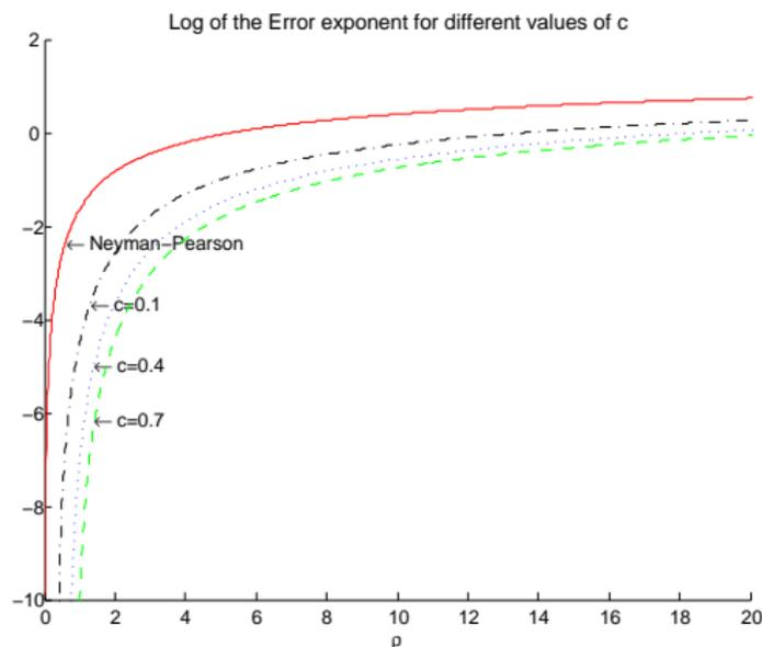
**Figure:** Computation of the logarithm of the Error Exponent for different values of  $c$  ( $\rho \geq \sqrt{c}$ ), and comparison with the optimal bound (Neyman-Pearson) obtained in the case where all the parameters are perfectly known.
