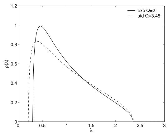
Spectrum of the exponentially weighted random matrix with n=1/2 and the spectrum of the standard random matrix with  $n\equiv N/T=1/3.45$ .
