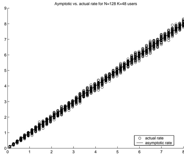
Figure 2: Comparison between the asymptotic and real rate for a system with  $N=128$  and  $K=48$
