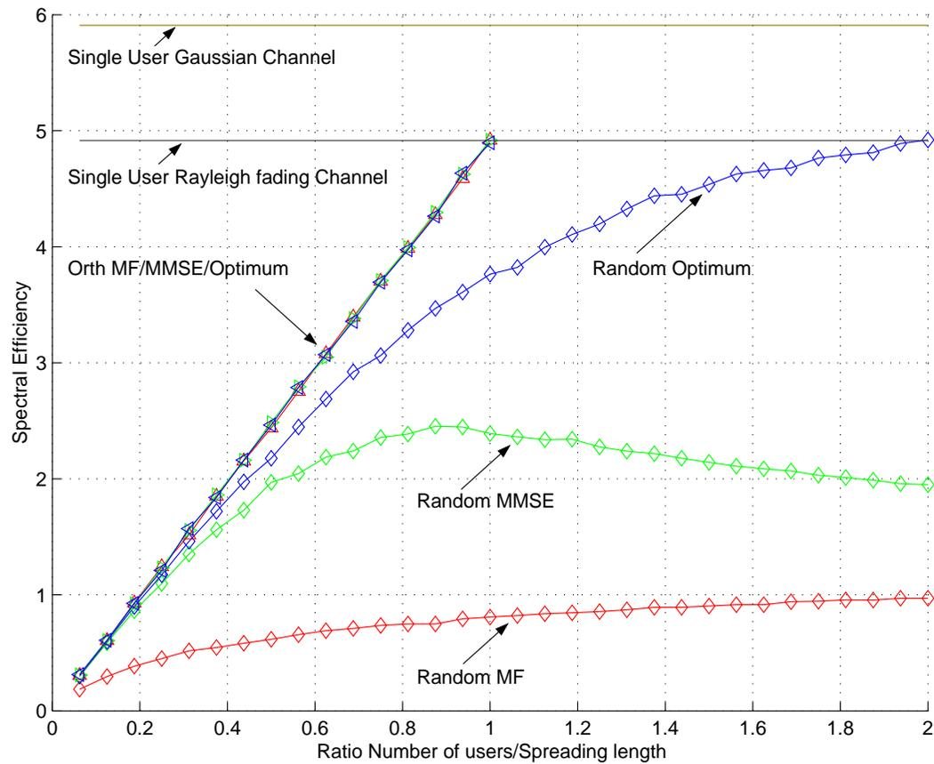
In a one-path channel, orthogonality gain is maximal.
