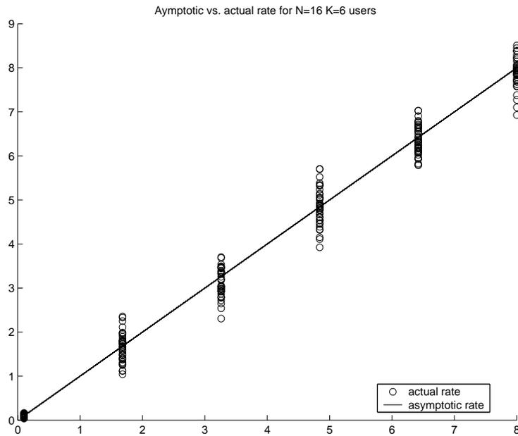
Figure 1: Comparison between the asymptotic and real rate for a system with  $N=16$  and  $K=6$
