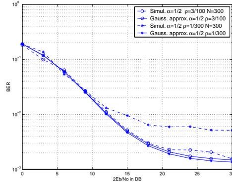
Fig. 3. BER for different values of  $N_s, N_h$ . Multi-path channels
