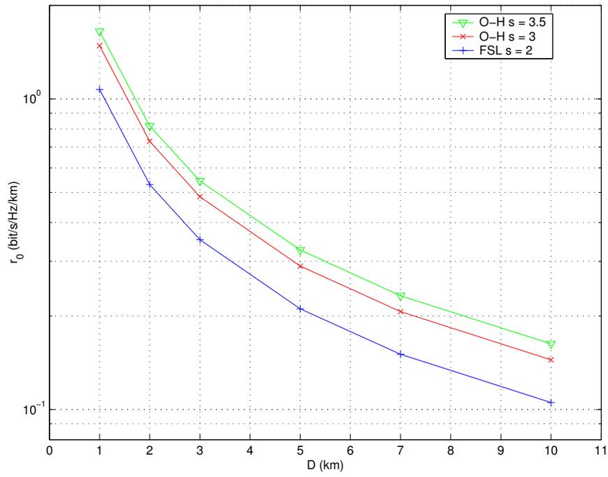
Fig. 9. Limit on the mean rate  $R_0$  vs. cell radius  $D$
