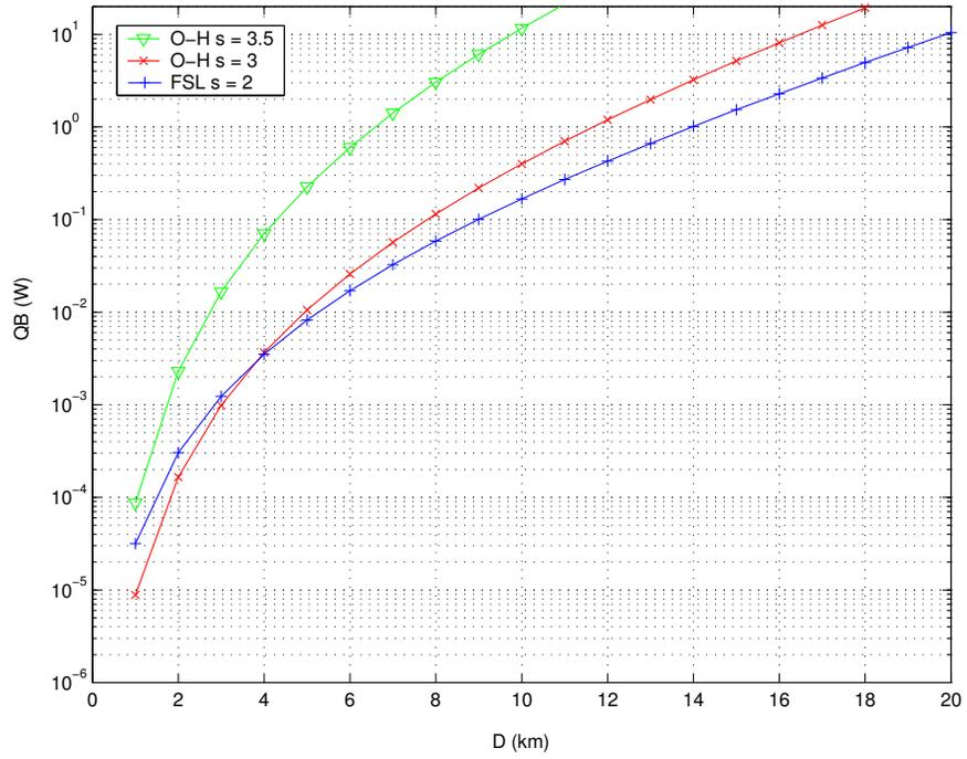
Fig. 4. Single cell context : required power vs. cell radius  $D$ ,  $\bar{r} = 0.2$  bit/s/Hz/km
