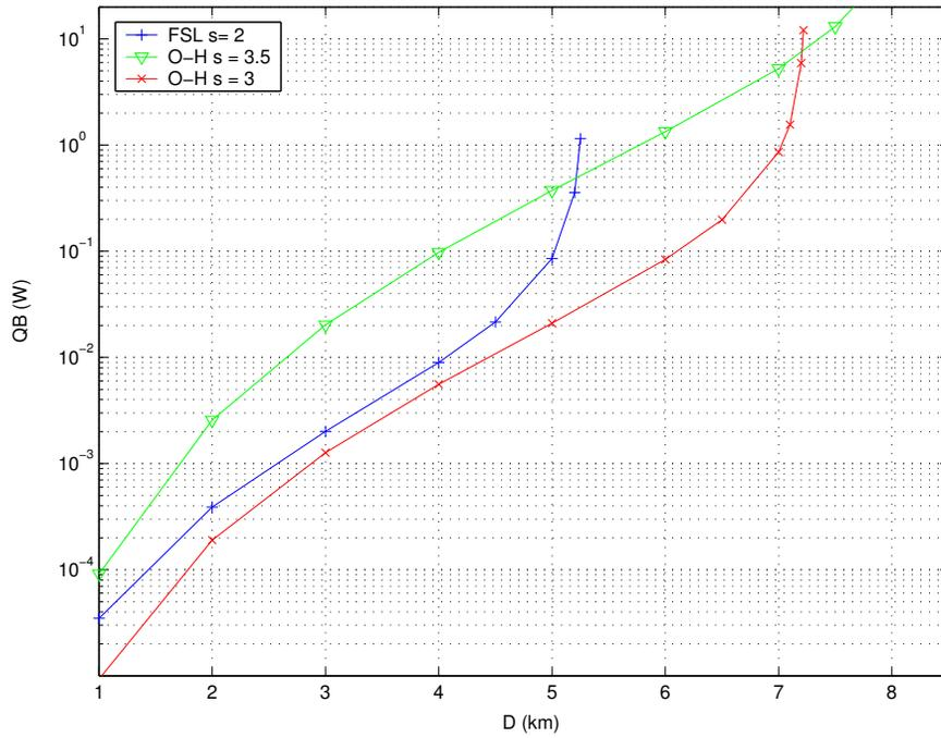
Fig. 6. Multi-cell context : required power vs. cell radius  $D$ ,  $\bar{r} = 0.2$  bit/s/Hz/km
