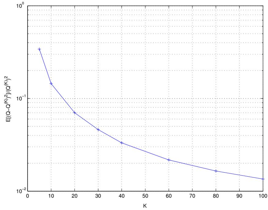
Fig. 3. Single cell context : normalized MSE between the total power  $Q$  required by the allocation algorithm and the power required in asymptotic regime  $Q^{(K)}$  vs. the number of users  $K$  (FSL model)
