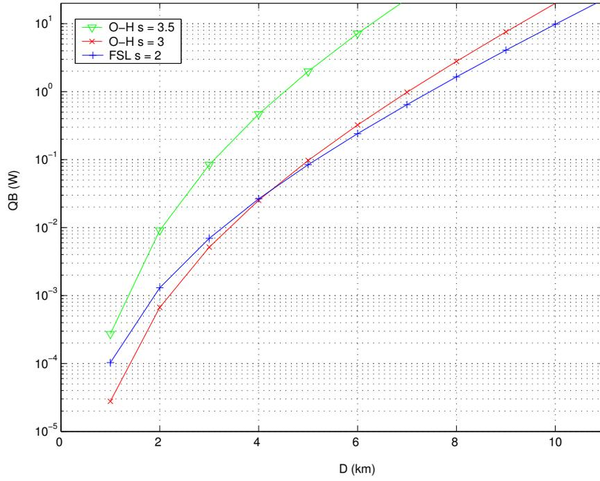
Fig. 5. Single cell context : required power vs. cell radius  $D$ ,  $\bar{r} = 0.5$  bit/s/Hz/km
