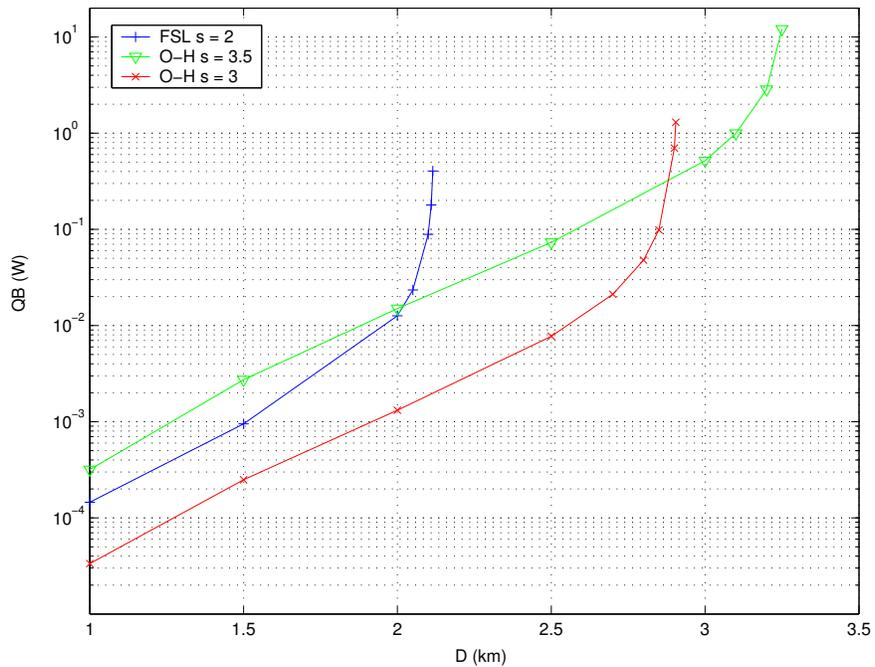
Fig. 7. Multi-cell context : required power vs. cell radius  $D$ ,  $\bar{\tau} = 0.5$  bit/s/Hz/km
