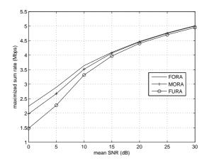
Figure 4: Maximized sum rate versus mean SNR for various resource allocation schemes
