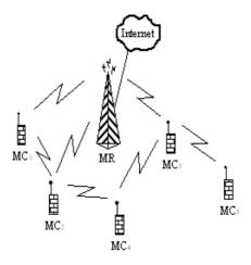
Figure 2: Illustration of a wireless mesh network
