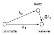
Figure 6: Illustration of a relay network operating in receiver cooperation mode.
