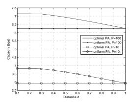
Figure 7: Maximized capacity vs. distance d for CDIT-based optimal power allocation and uniform power allocation.
