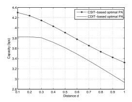
Figure 8: Maximized capacity vs. distance d for CDIT-based optimal power allocation and CSIT-based optimal power allocation
