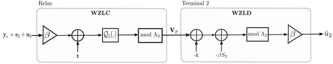
Fig. 3. WZ Lattice Coding and Decoding at T<sub>2</sub>
