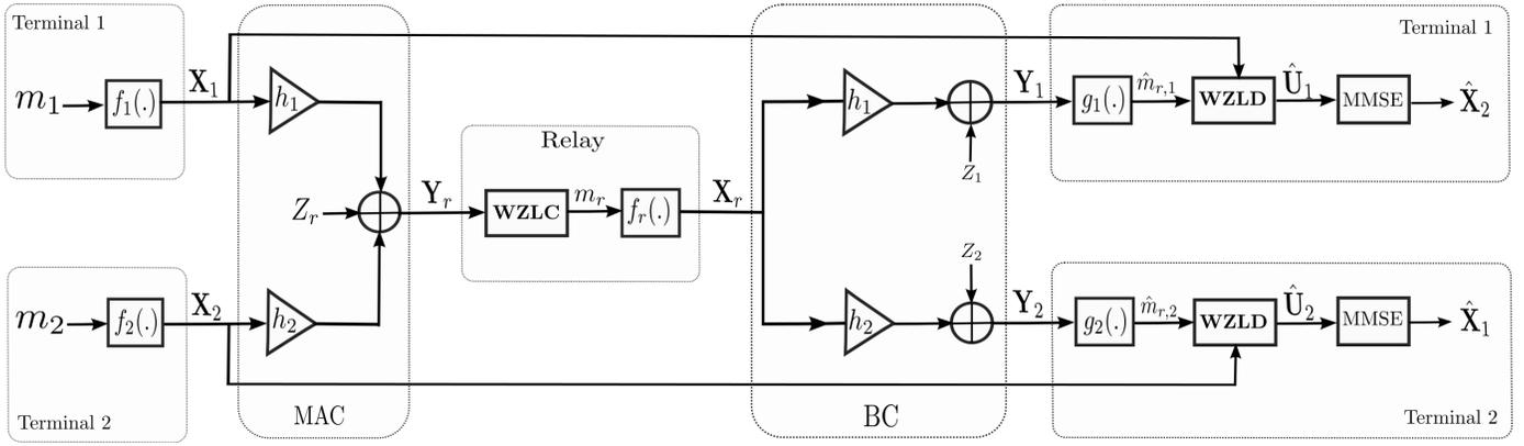
Fig. 2. Channel Model for TWRC
