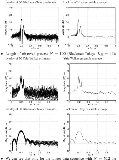
• We can see that only for the longer data sequence with N = 512 the resolution of the estimates are comparable. Clearly, for N = 100 the estimate based on an AR-model provides much better frequency resolution for the sinusoidal components than the Blackman-Tukey method.
