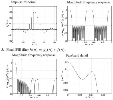
6. H(z) in the IFIR realization has an overall length of 35 coefficients. On the other hand we obtain from (4.73) an estimated length of 65 coefficients for the direct form implementation.
