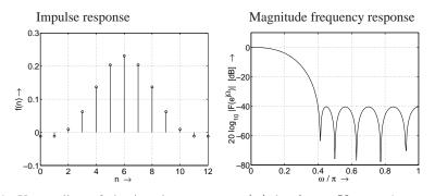
4. Upsampling of the impulse response g(n) by factor  $K = 4 \rightarrow g_1(n) \frown G(e^{jK\omega})$ :
