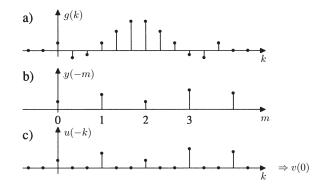
$\Rightarrow$  The output sample v(0) is obtained by multiplication of g(n) with u(-n), where a lot of zero multiplications are involved, which are inserted by the upsampling operation.
