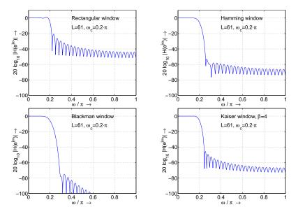
**MATLAB-command** for windowed linear-phase FIR design: fir1
