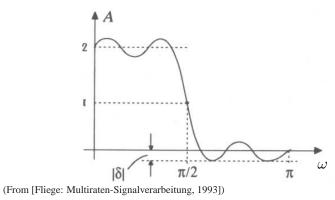
$\Rightarrow$  Single zeros on the unit-circle are converted to double zeros  $\rightarrow$  factorization into two filters is now possible
