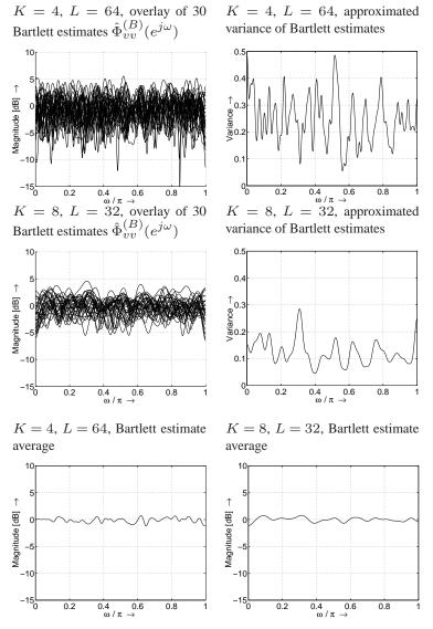
• Here, the input signal consists of two sinusoids in white Gaussian noise
