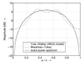
$\rightarrow$  Blackman-Tukey estimate, which makes no assumption about the process, yields a better estimate of the power spectrum compared to the model-based Yule-Walker approach.
