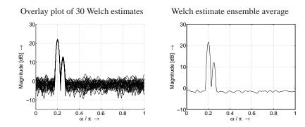
Compared to the Bartlett estimate for the same example above the use of the Hamming window reduces the spectral leakage in the estimated power spectrum.
