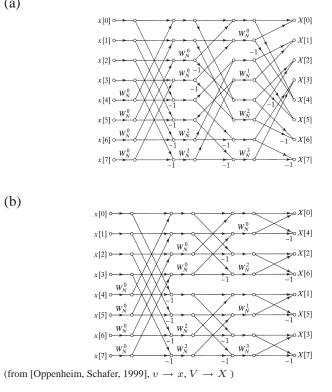
The flow graph in (a) has the disadvantage, that it is a *non-inplace* algorithm, because the butterfly-structure does not continue past the first stage.
