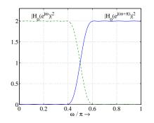
$\rightarrow$  It can be easily shown that the power-complementary property also holds for  $h_1(n)$ ,  $f_0(n)$ , and  $f_1(n)$ .
