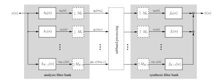
Subband processing: Quantization (wordlength reduction)  $\rightarrow$  coding, (adaptive) filtering  $\rightarrow$  equalization, ...
