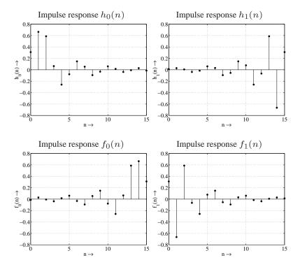
Filter in orthogonal two-channel filter banks have an even number of coefficients since T<sub>Z</sub>(z) = H<sub>0</sub>(z) H<sub>0</sub>(z<sup>-1</sup>) Example:
