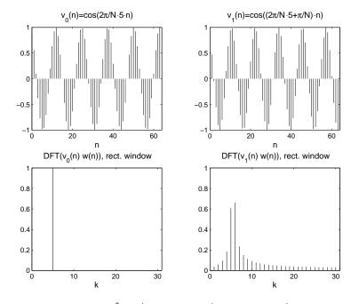
• Left hand side:  $\hat{V}_0(e^{j\omega_k}) = V_0(e^{j\omega_k}) \circledast W(e^{j\omega_k}) = 0$  for
