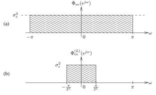
Gain in (5.45) can also be used for reducing the quantizer wordlength while keeping the SNR constant:
