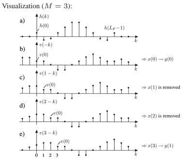
$\Rightarrow$  Multiplication of h(n) with v(1-n) and v(2-n) leads to the results x(1) and x(2) which are discarded in the decimation process  $\rightarrow$  these computations are not necessary.
