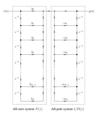
Another realization can be obtained by exchanging the order of the all-pole and all-zero filter. Then, the difference equation for the all-pole section is
