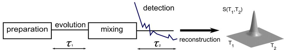
$$Y(\tau_1, \tau_2) = \iint (1 - \gamma e^{-\tau_1/T_1}) S(T_1, T_2) e^{-\tau_2/T_2} dT_1 dT_2 \xrightarrow{\text{discretization}} \begin{cases} \mathbf{Y} = \mathbf{K}_1 \mathbf{S} \mathbf{K}_2^t \\ \mathbf{y} = \mathbf{K} \mathbf{s} \end{cases}$$
