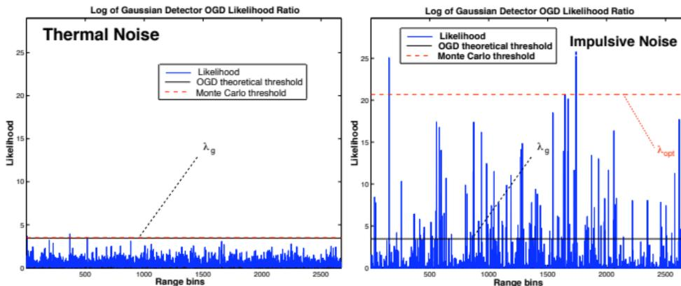
FIGURE : Failure of the OGD - Adjustment of the detection threshold - K-distributed clutter with same power as the Gaussian noise
